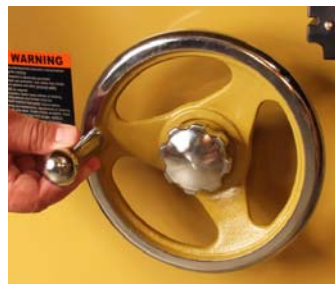
The spindles (left) are retained with a tough drawbar and locking nut. Spindle height changes are done using the large-diameter cast iron handwheel (right) fitted with a spinner handle.
