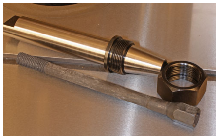
The spindles (left) are retained with a tough drawbar and locking nut. Spindle height changes are done using the large-diameter cast iron handwheel (right) fitted with a spinner handle.
