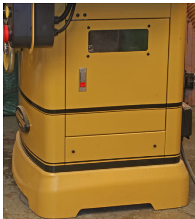
The cast iron base and retractable casters make moving this machine both mobile and rock steady when in use.
