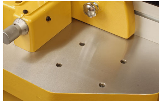
Both rear corners of the table are pre drilled and tapped to accept our popular feeder systems
