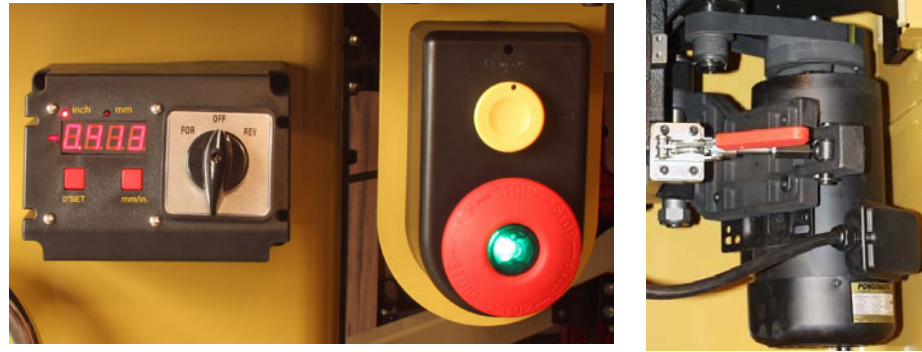
The controls (left) are grouped where they are in easy reach of the operator. The powerful motor (right) is easily accessible through the large side door. Changing spindle speeds is fast and tool-free.
