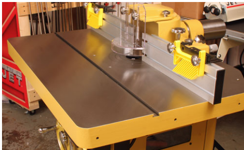
The huge cast iron table (left) makes working with large pieces safe and accurate. The cast iron insert rings (right) let you size the opening to best fit the cutter being used.
