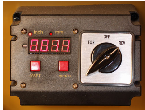
The digital spindle height display makes super accurate height changes dead-on simple.
