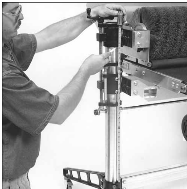
Fig. 18. Comparing brush support casting heights.
