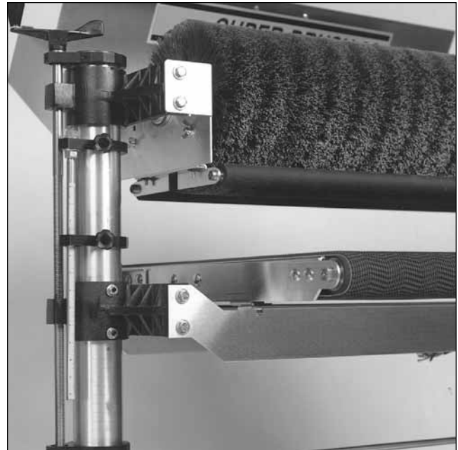
Fig. 16. Height controls on outboard side.
