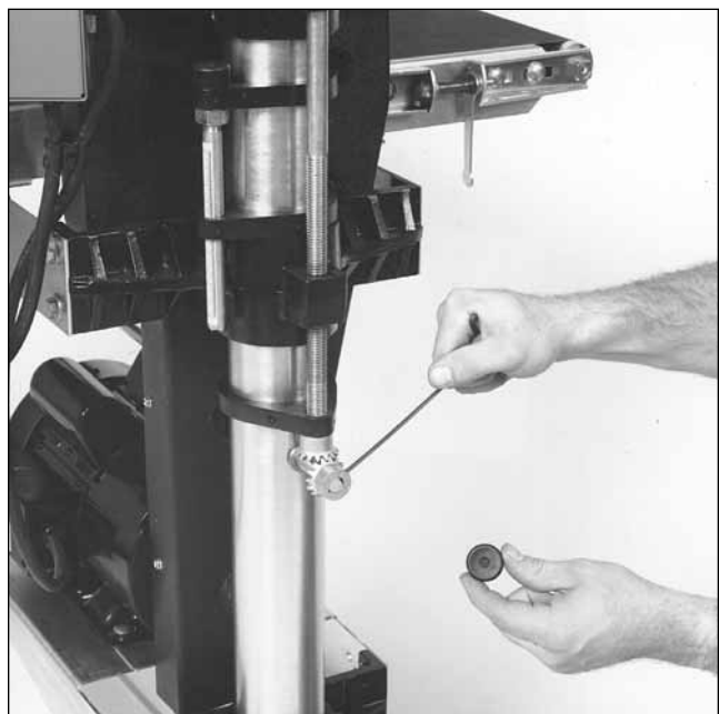
Fig. 14. Adjusting miter gears for proper mesh.
