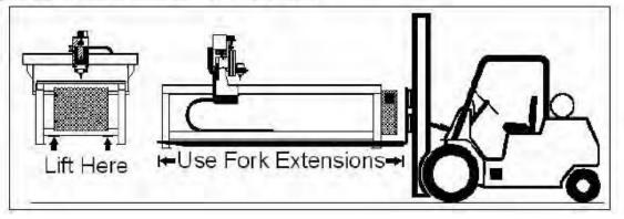
Warning: CNC equipment may not be balanced. Use caution when moving or unloading so as not to damage CNC equipment, fork lift, or operator. See picture.
