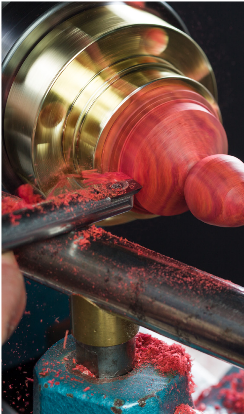
Square tool shown in photo. Centerline alignment applies to all Ultra-Shear Woodturning Tools.
