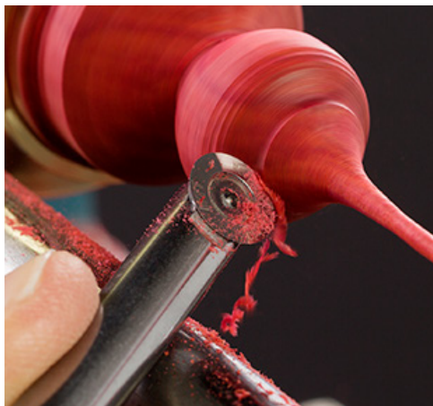
Round insert shown in photo. Technique applies to both square and round Ultra-Shear Woodturning Tools.
