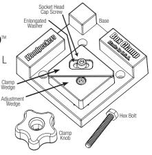
The Box Clamp can be used in "Fixture" or "Hand Clamp" mode. In both cases the clamp works by wedging the material into the fixed stops of the base. In Hand Clamp mode, you'll use a knob from the backside of the clamp. In Fixture mode you'll tighten the clamp using a socket head cap screw and hex key from the top.
