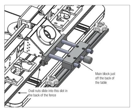
Before attaching the Micro Adjust to the back of your fence, slide the fence toward the back of your router table so the main block is positioned just off the table. Now align the front two oval nuts with the slot toward the bottom, back of the fence. With these two oval nuts fully engaged in the slot, slide the entire Micro Adjust assembly until it's approximately centered with the fence. Just barely tighten the screws.
