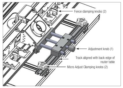
Once the fence Micro Adjust is approximately centered on the fence, slide both it and the fence toward the center of the table. During this step you need to align the bolt heads below the track with the track slots in the table.
