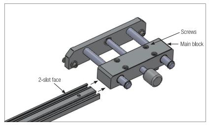
Attach the main block to the top of the track (2-slot face) by sliding all four oval nuts into the slots. With the main block approximately centered, tighten all four screws.
