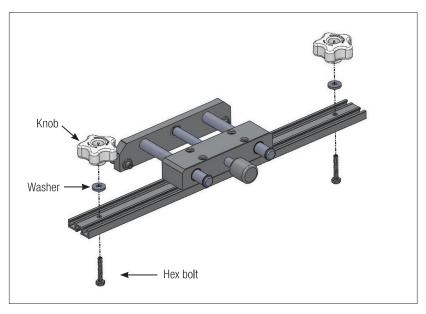
Now insert the two hex bolts up through the two holes in the track. First slip a nylon washer over each bolt then loosely start each knob.
