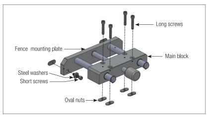
Begin by installing the (4) long screws down through the main block. Loosely start the oval nuts from the bottom. Next install the (2) short screws and washers through the fence mounting plate as shown. Loosely start oval nuts on these two as well.
