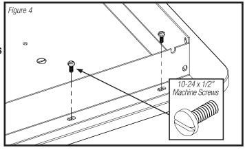
For other brands of stands or a shop built stand drill & tap the **Phenolic Router Table** as needed, being careful not to drill completely through the table.
