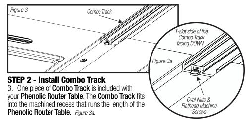
Place an **Oval Nut**, smooth side down, aligned with one of the holes in the machined recess. From underneath the table, insert a **Flathead Machine Screws** through the table and thread loosely onto the **Oval Nut**. Repeat for all holes in the recess.
