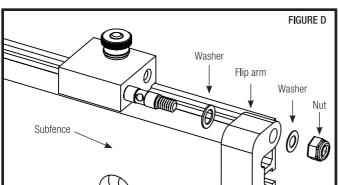
1. Use a 7/16" wrench to remove the nut holding the flip arm to the body. Then remove the first nylon washer, the flip arm and the second nylon washer. FIGURE D.
