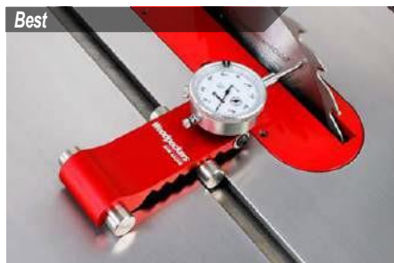
A dial indicator on a dedicated tool, like this Saw Gauge sold by Woodpeckers®.
