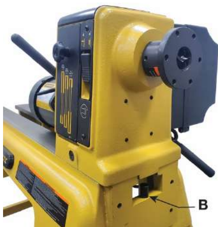
Figure 8-2: Outboard Turning Position
